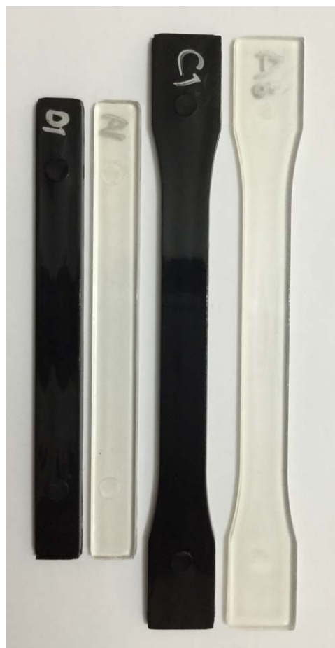
Figure 2. The shape of fabricated samples after injection molding process. [Color figure can be viewed in the online issue, which is available at wileyonlinelibrary.com .]
